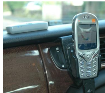
Figure 20: Illustration of car kit with phone holder and Bluetooth GPS device on top of instrument panel.
